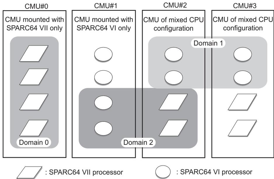
A mix of SPARC64 VI and SPARC64 VII processors can be mounted on a single CMU, as shown in CMU#2 and CMU#3 in FIGURE 4-6. And a single domain can be configured with a mix of these SPARC64 processors, as shown in Domain 2 in FIGURE 4-6.
