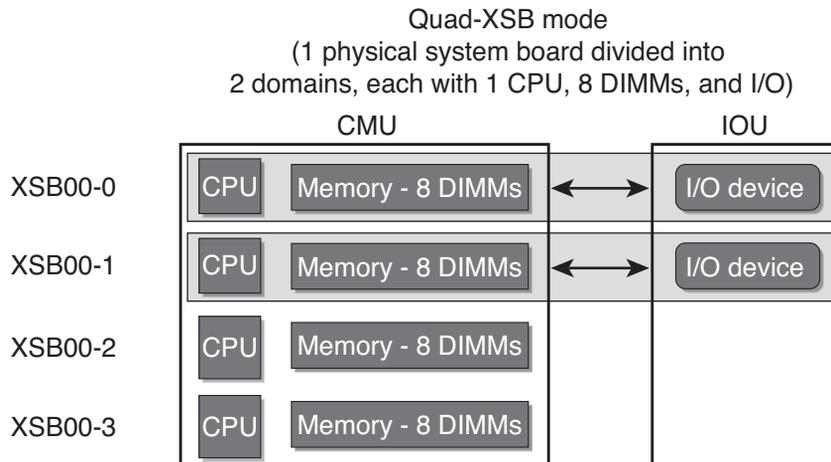
**FIGURE 4-4** A Physical System Board in Quad-XSB Mode on a High-End Server
