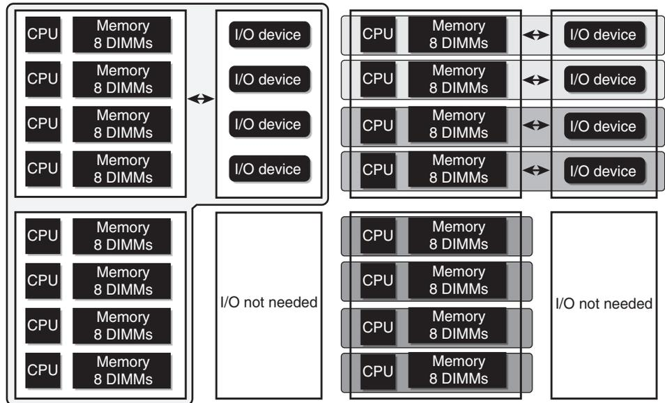
The Solaris OS is installed on a per-domain basis. In the configuration shown in [FIGURE 4-5](#), there would be three Solaris images, one for each domain.
