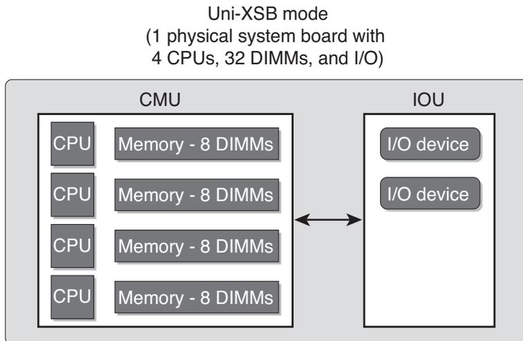
**FIGURE 4-2** A Physical System Board in Uni-XSB Mode on a High-End Server
