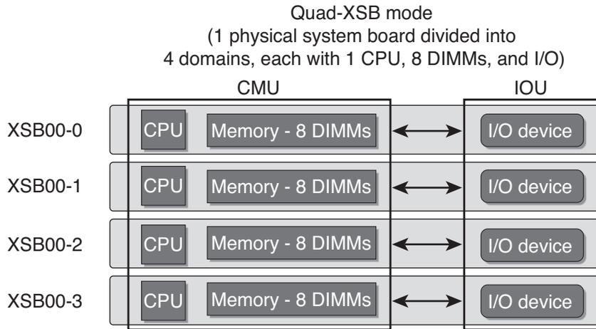
A domain consists of one or more XSBs. Each domain runs its own copy of the Solaris OS. A domain must have, at a minimum, 1 CPU, 8 DIMMs, and I/O.
