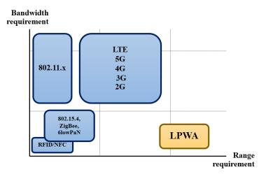
Figure 1 Show graph of bandwidth required and range capability of wireless technology
