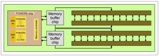
Figure 2-5 Power 520 4.2 GHz memory socket layout view
