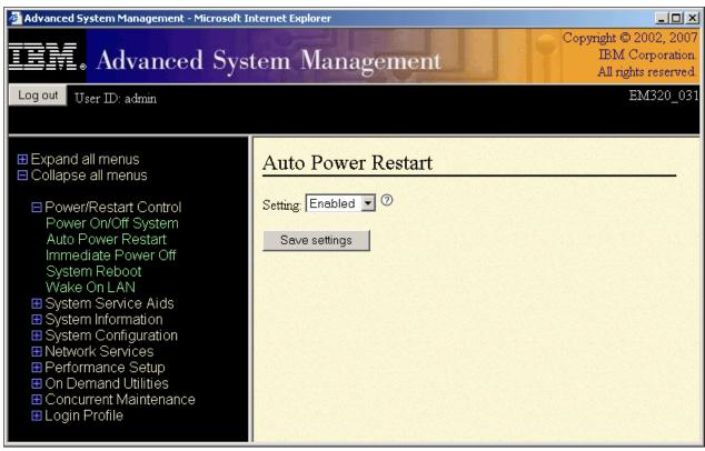
Figure 4-2 ASMI Auto Power Restart setting
