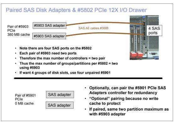
Figure 2-33 SAS Disk Adapters and #5802 PCIe 12X I/O Drawer
