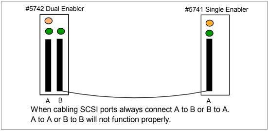
Figure 2-14 Logical cabling view between EXP24 enabler (repeater) adapters
