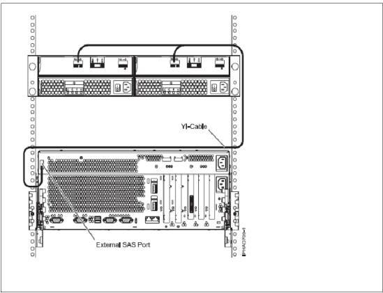
Figure 2-22 Single enclosure attached with YI cable to external SAS port
