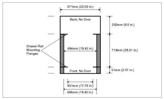
Figure 1-9 Top view of non-IBM rack specification dimensions
