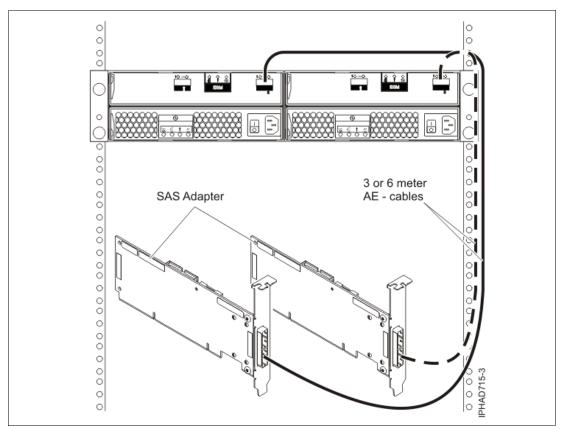
Figure 2-26 Schematic for HA configuration on EXP12S
