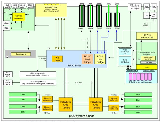
Figure 2-1 Power 520 logic data flow (8310 backplane)
