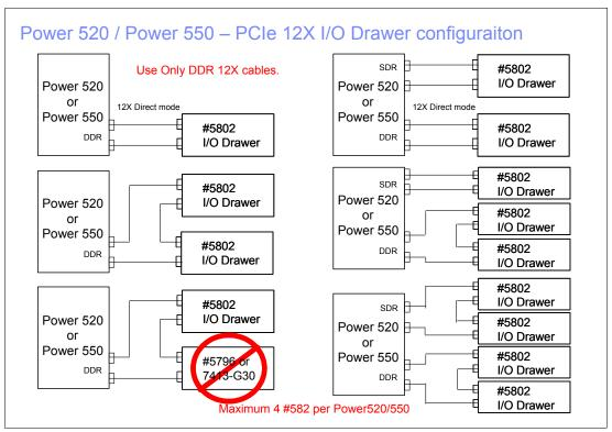
Figure 2-31 PCle 12X I/O drawer loop configurations with Power 520 and Power 550
