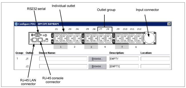
Figure 1-8 Power Distribution Unit plus example
