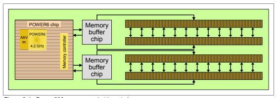
Figure 2-4 Power 520 memory socket layout view
