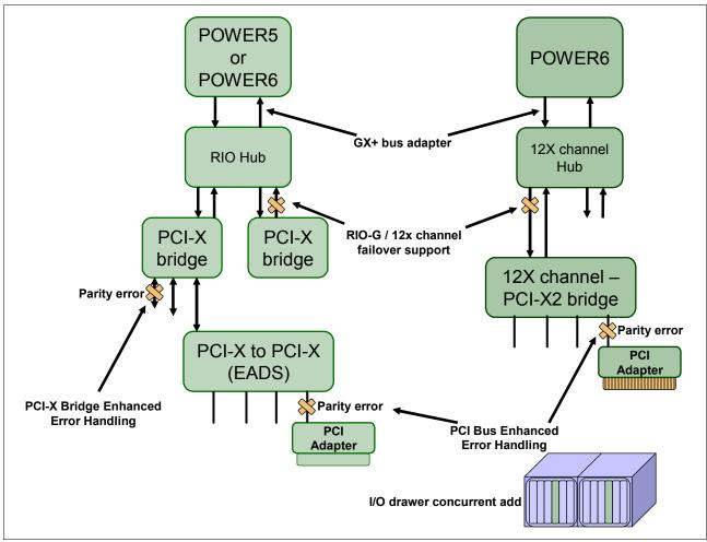
Figure 4-5 PCI error recovery
