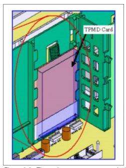
Figure 2-3 Thermal power management device (TPMD) card
