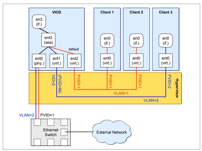
Figure 3-3 Architectural view of a Shared Ethernet Adapter
