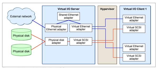
Figure 3-2 Architectural view of the Virtual I/O Server
