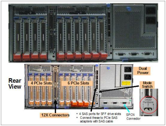
Figure 2-28 Rear view #5802 PCIe 12X I/O drawer
