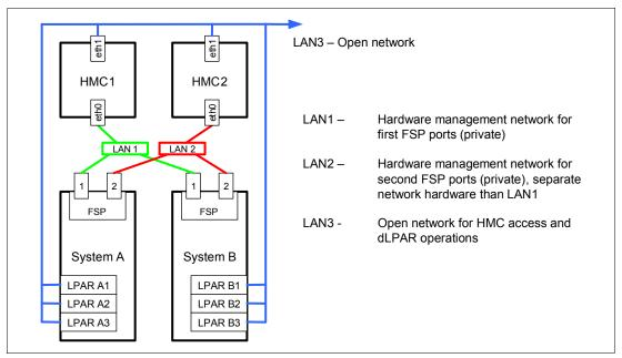
Figure 2-36 Highly available HMC and network architecture
