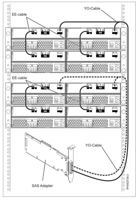
Figure 2-21 Maximum attachment of EXP 12S on one adapter
