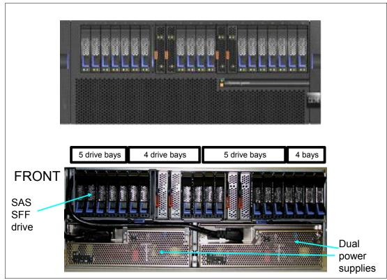
Figure 2-27 Front view #5802 PCIe 12X I/O Drawer
