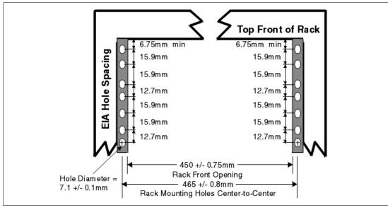
Figure 1-10 Rack specification dimensions, top front view
