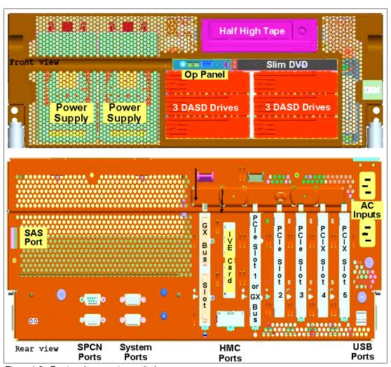
Figure 1-3 Front and rear system unit views
