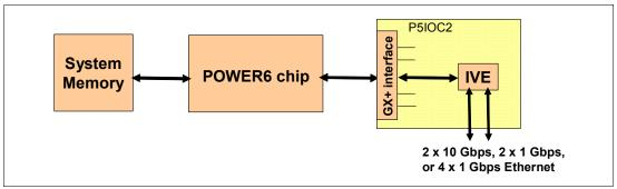
Figure 2-9 IVE system placement
