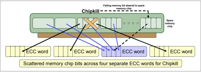
Figure 4-3 Memory protection capabilities in action
