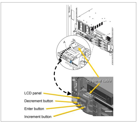
Figure 2-37 Operator control panel physical details
