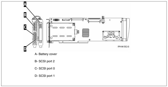
Figure 2-16 EXP 24 ports and batter cover
