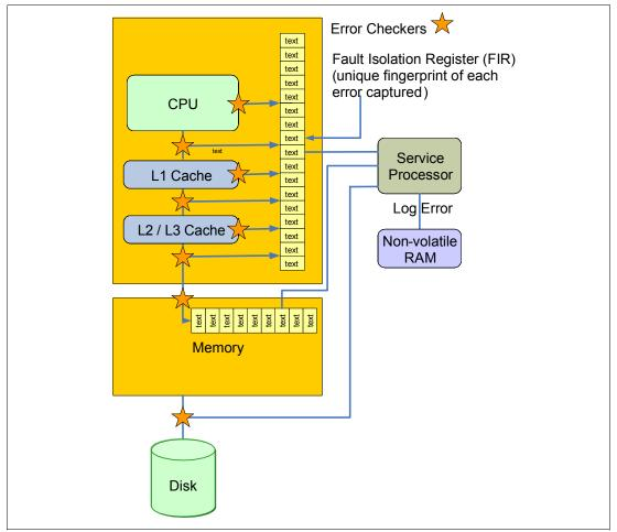
Figure 4-6 Schematic of an FIR implementation
