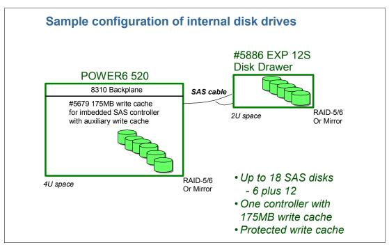
Figure 1-5 EXP 12S attached to the system unit example
