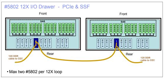
Figure 2-30 Two #5802 PCIe 12X I/O Drawers on a loop
