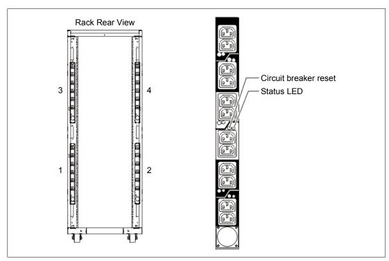
Figure 1-7 PDU placement and PDU view
