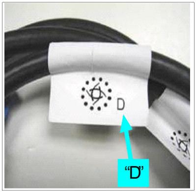
Figure 2-32 New 12X DDR connection cable
