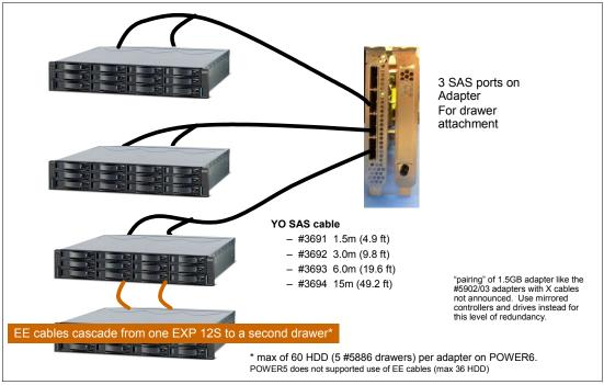
Figure 2-24 Schematic for 5904 connectivity to EXP12S
