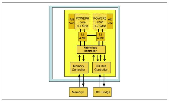
Figure 2-2 POWER6 processor
