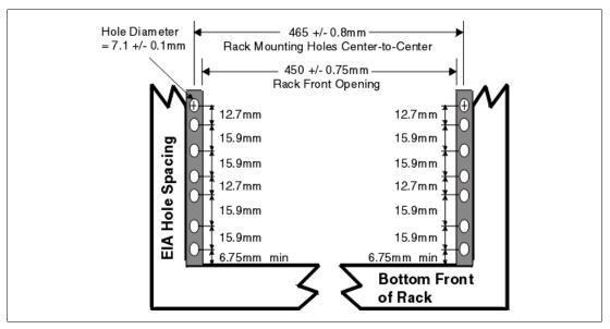
Figure 1-11 Rack specification dimensions, bottom front view
