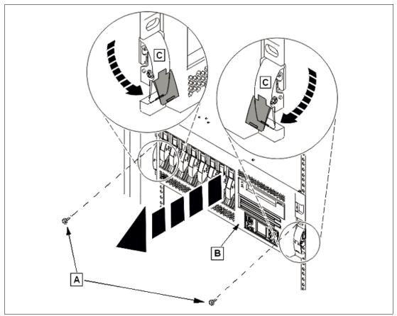
Figure 2-39 Pull the Power 520 to the service position
